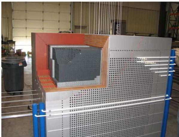
B Reactor model with pile cutaway
