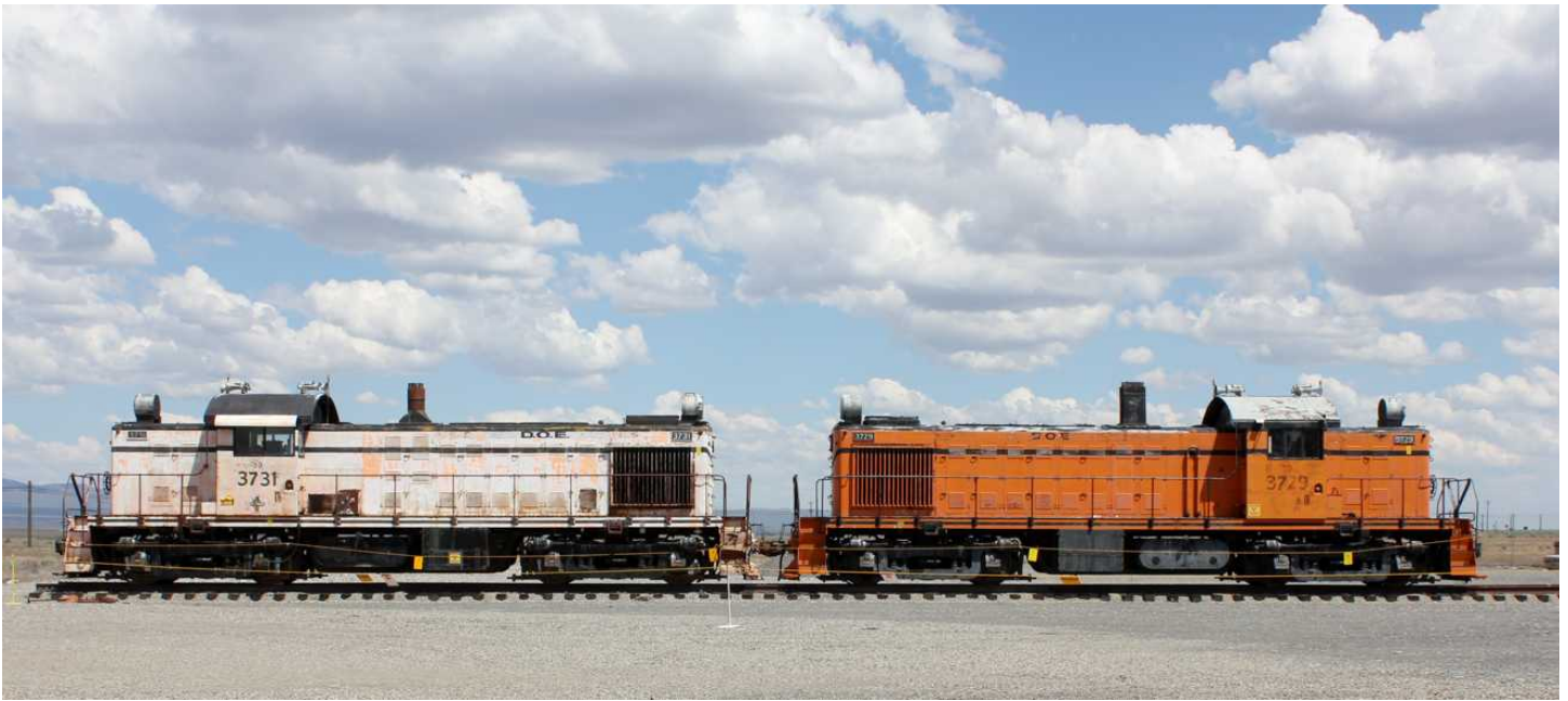
These locomotives were used to move shielded fuel transfer cask and rail cars between Hanford reactors and chemical processing and separations plants. They now are on display at B Reactor. Photo by Bob Horgos
