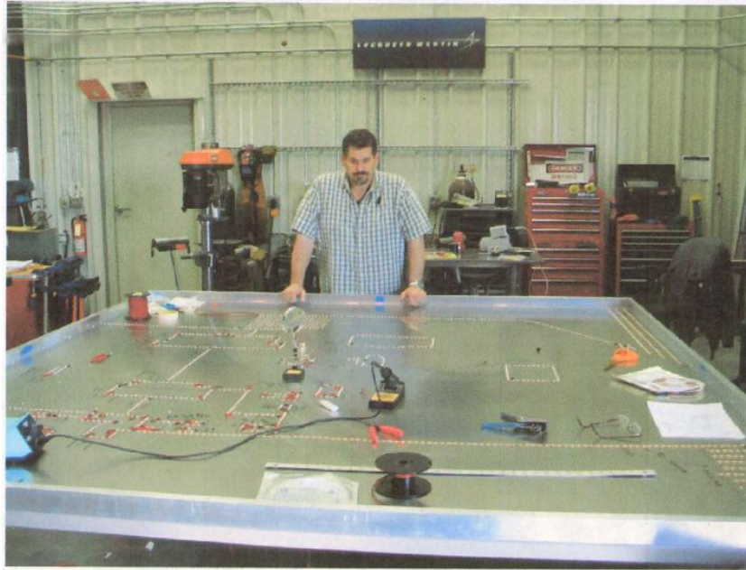
The base 8-ft. X 8-ft. model layout with wiring for lights to be used for identifying individual site facilities. Lynn Ver Steeg of Lockheed-Martin is observing.
