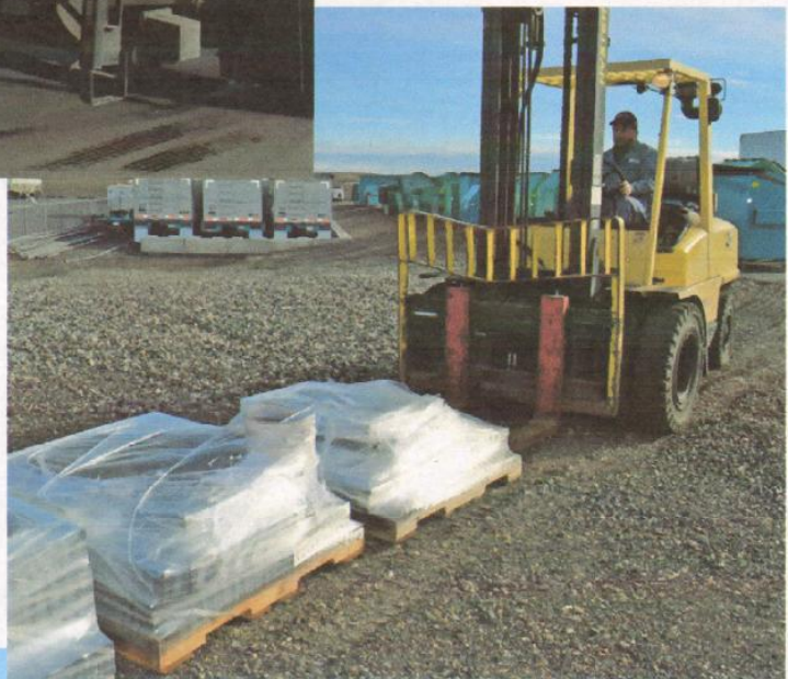
A heavy-duty fork-lift was used to move the dense graphite .
